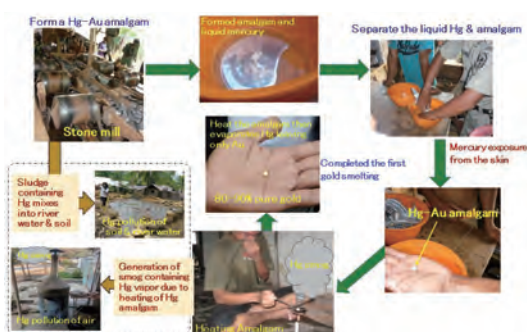
Fig. 1 Hg amalgamation process and pollution related to ASGM.
