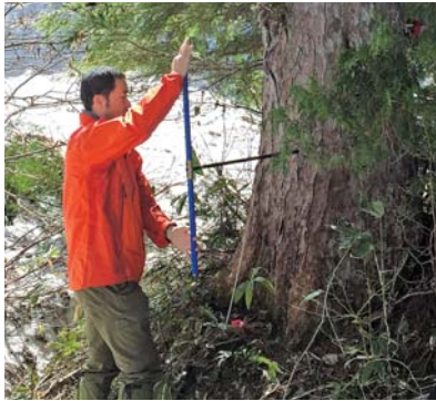
Photo 1 Collection of tree-ring cores using an increment borer
