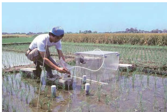
Using the closed chamber technique to monitor greenhouse gas emissions from rice paddies.
